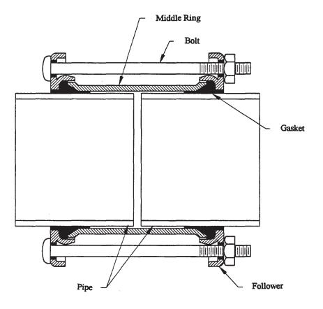
Figure 11-1. Flexible Coupling (Source: Dresser Industries, Inc., fistyle 38 Dresser Couplings for Steel Pipe Sizes, Sizes and Specifications,f1Form 877-C Rev. 1095)
